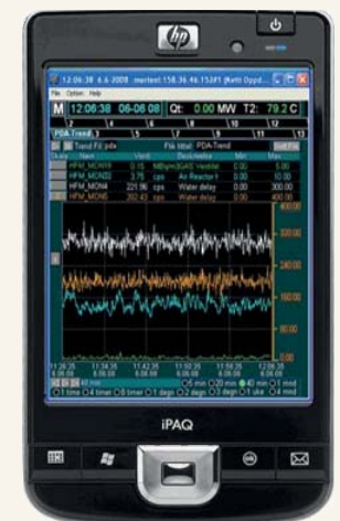
Trend curves on mobile device, Halden Reactor
