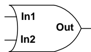
Figure 4 An OR-gate can be realized using a graphic class. The class is defined with two input terminals and one output terminal. The input terminals can be assigned to some application variables, in order to illustrate some logic state of an application
