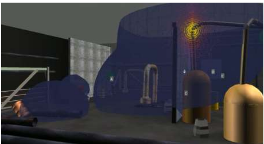
Figure 3.3 View Dependent smooth isosurfaces in combination with a point cloud, showing the boundary between the radiation level at the current location and the next level.
