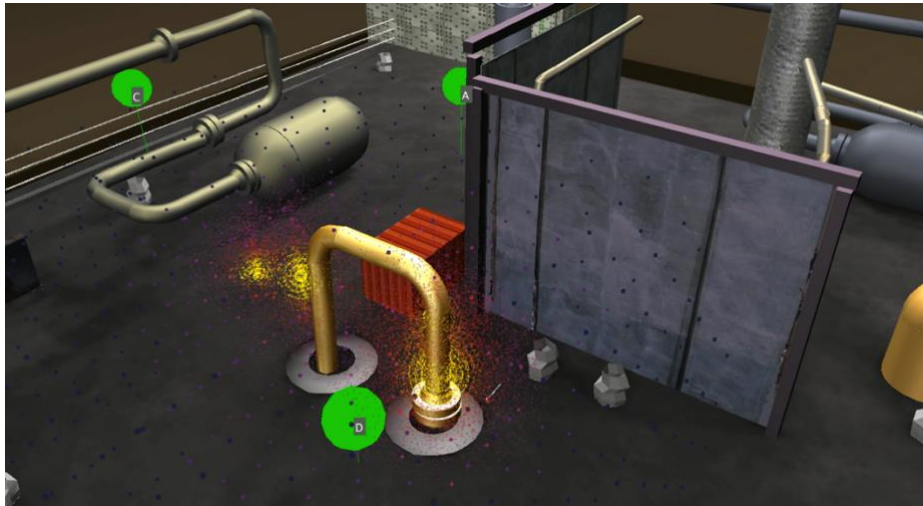
Figure 3.1 Point cloud with Density Proportional to Radioactivity Level.
