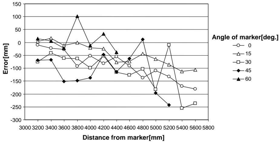
Figure 4: Errors of position estimation. (Single marker)
