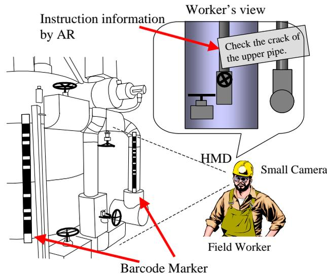
Figure 1: Image of Barcode marker and Tracking System.
